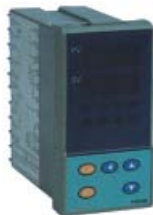
LS-908 Outlook Dimension 48X96X100mm Hole Dimension 45 ±1 X 91 ±1
