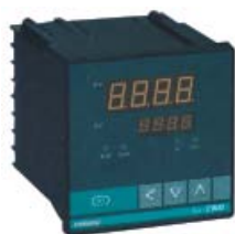
LS-C900 Outlook Dimension 96X96X113mm Hole Dimension A 92 +0.8 B 92 +0.8
