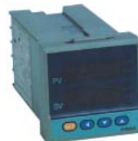
LS-904 Outlook Dimension 48X48X100mm Hole Dimension 45 ±1 X 45 ±1
