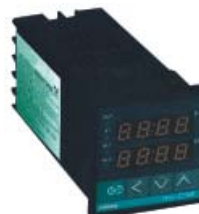
LS-C100 Outlook Dimension 48X48X108mm Hole Dimension A 45 +0.6 B 45 +0.6
